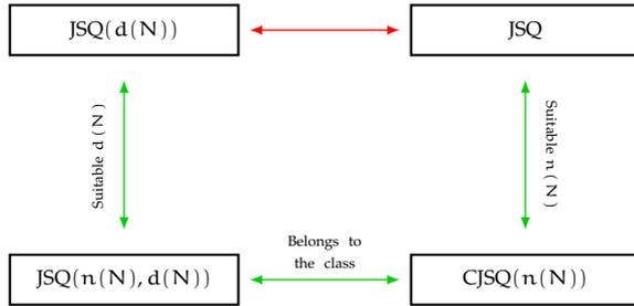
**Figure 5:** Asymptotic equivalence relations. The equivalence structure is depicted for various intermediate load balancing schemes to facilitate the comparison between the  $JSQ(d(N))$  scheme and the ordinary JSQ policy.
