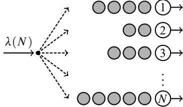
**Figure 2:** Tasks arrive at the dispatcher as a Poisson process of rate  $\lambda(N)$ , and are forwarded to one of the  $N$  servers according to some specific load balancing algorithm.
